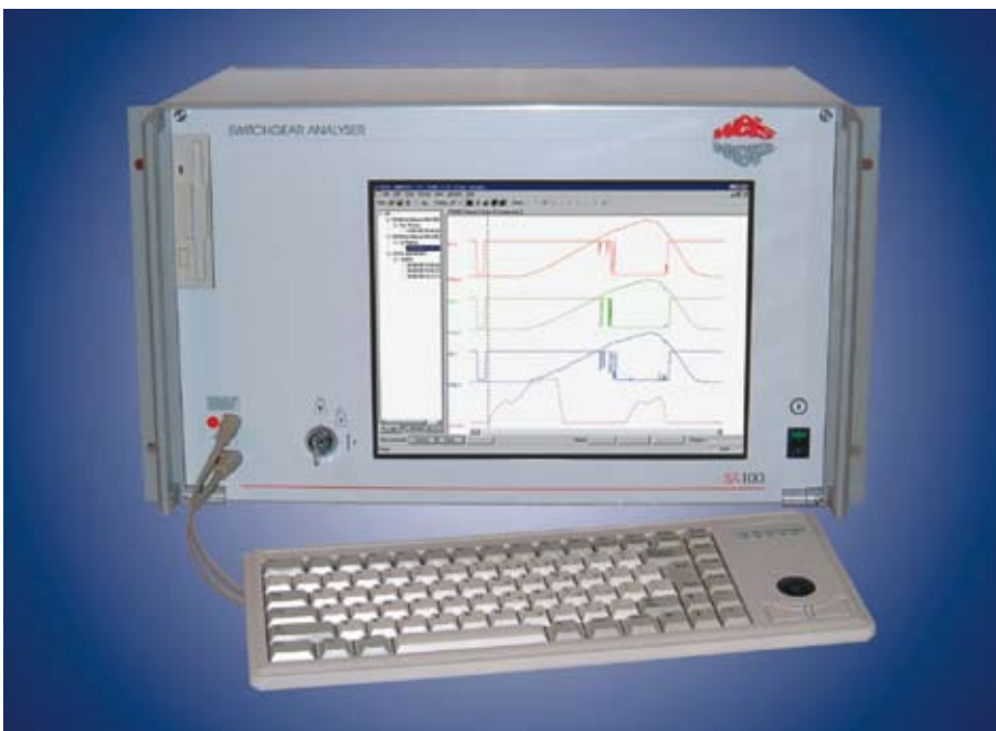
The Weis SA 100 is a rugged portable analysis system for high voltage circuit breakers, providing precise data on the condition of switch contacts without the need to open the circuit breaker housing (photo: Weis)
