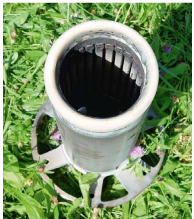
The moving outer contact also shows considerable signs of wear (photo: Weis)
