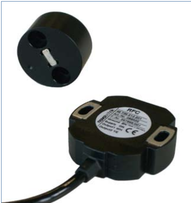
A magnetic angle sensor in which the sensor and the position marker are designed as separate components (RFC 4800). The position-marker with incorporated magnet is simply mounted on the rotating shaft. With the CleanCab System as well, this simplifies the integration, as no shafts had to be centred (Photo: Novotechnik)
