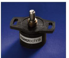
Designed for industrial, materials handling, robotic, overhead doors and automotive drive-by-wire applications, RSM 2800 tracks and permanently stores shaft rotation as well as position when power is lost. Upon restoration of power, it detects the new position, calculates the difference to automatically provide accurate position and count. Position and count information can be retained without power for years.
