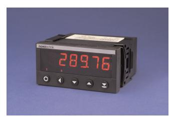
Operated either by five buttons on the front panel or remotely via serial interfaces, the MAP 4000 provides isolated RS 232 or RS 485 outputs. There are two programming levels available: a code protected configuration menu and a user menu to prevent end user errors.
