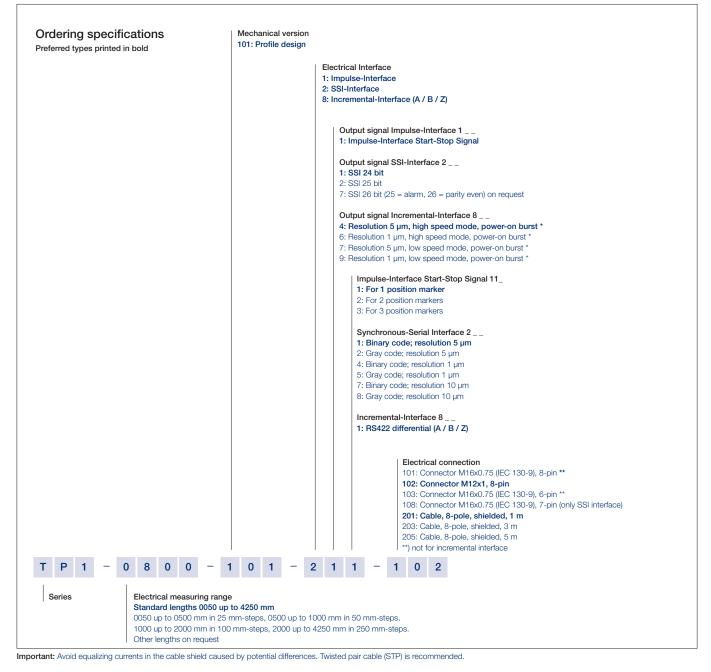
\*) Power-on burst: The burst output is triggered by switching on the power supply. The current sensor position as an absolute value is put out as an incremental pulse sequence with the selected frequency of 156 kHz (high speed mode) or 78 kHz (low speed mode). The number of pulses corresponds to the distance to the zero point in the set effective direction and resolution.
