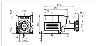
Signal conditioner integrated in mating plug connector with 24 V and standard output signals. MUW-200: range and zero point not adjustable MUW-250: range and zero point adjustable Detailed data see separate data sheet.
