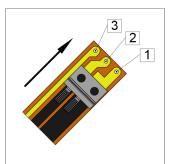
Direction of output characteristic when moving in direction of the electrical connection: increasing: supply voltage Ub at connection 1 falling: supply voltage Ub at connection 3
