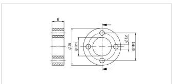
Ring position marker for fixation with screws M3
