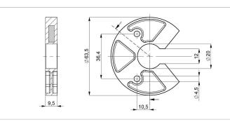
U-shaped position marker for fixation with M4 screws
