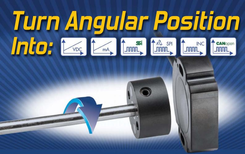
RFC 4800 Series sensors measure angular rotation using a magnet attached to your application's shaft. Since they're absolute sensors, they keep measuring even if you lose power and report the correct position when power is restored. Voltage, current and digital output options provide design flexibility to choose the interface that works best for you.
