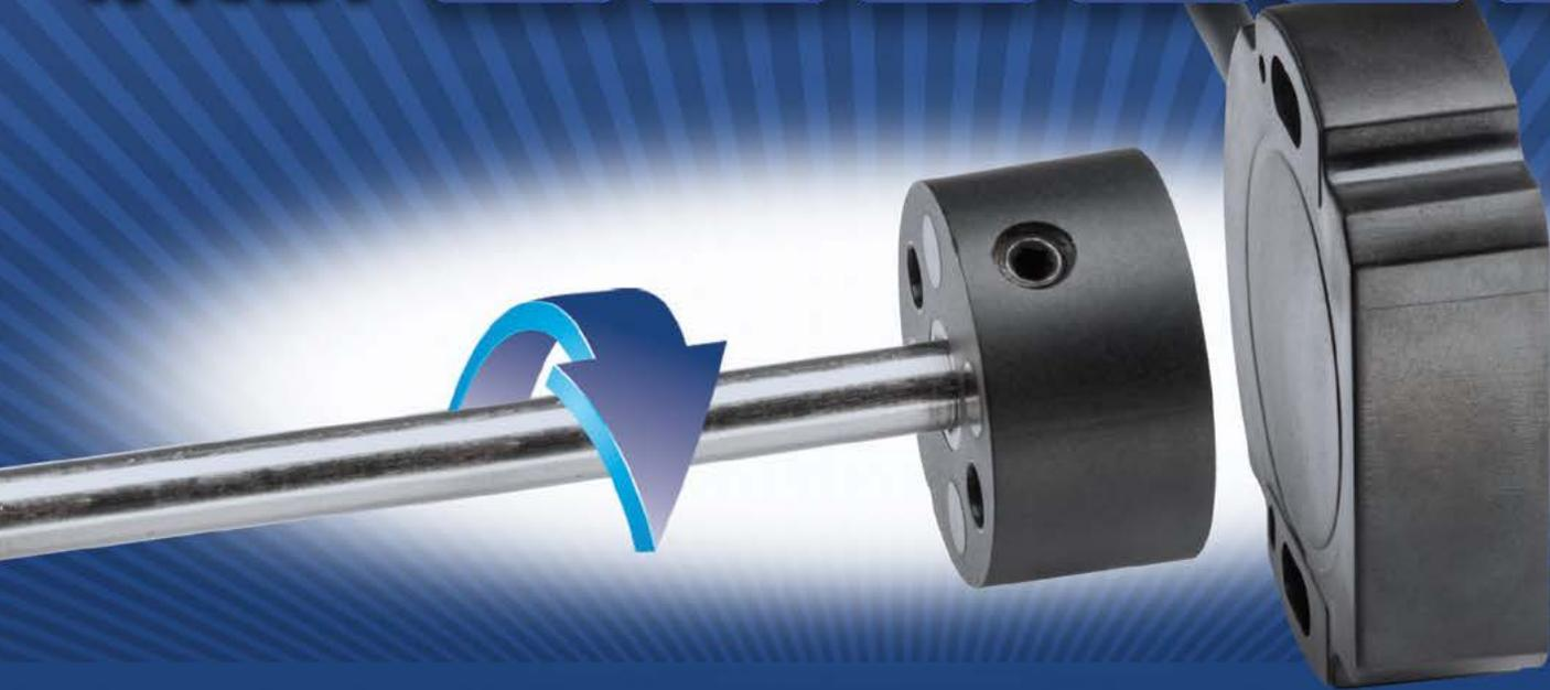
RFC 4800 Series sensors measure angular rotation using a magnet attached to your application's shaft. Since they're absolute sensors, they keep measuring even if you lose power and report the correct position when power is restored. Voltage, current and digital output options provide design flexibility to choose the interface that works best for you.
