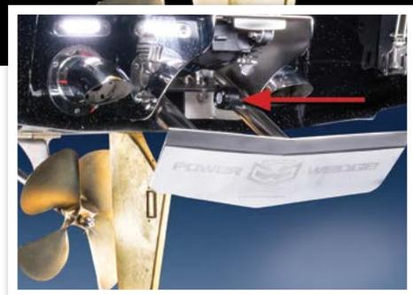
**Here's where the Novotechnik magnetic sensor measures angle.**
