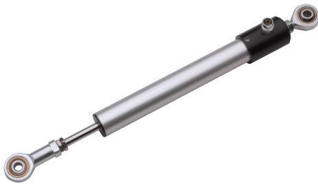
TX2 Series sensors are available from stock in eight stroke lengths from 25 to 300 mm. These sensors also feature compact size with mechanical lengths from 88 to 374 mm, measured on center of pivot heads and a housing diameter of 18 mm.
