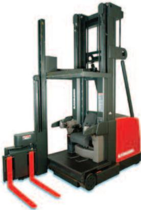
The new Swing-Reach trucks can elevate up to 45 feet (12.8 m), can handle loads up to 60 inches (152.4 cm) deep or 108 inches (274.32 cm) wide, and can operate in aisles as narrow as 66 inches (167.64 cm). The mini mast can be moved at a lateral speed of up to 8 inches per second. Raymond has hundreds of 9000 series trucks operating at customer sites.
