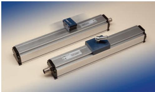
The TP1 Series is plug-in compatible with other similar sensors and is offered in standard measurement ranges of 50 to 4,500 mm. Other key specifications include update rate of 62  $\mu$ sec, absolute linearity to within  $\pm 0.02$  % of F.S, 16-bit resolution and sealed to meet the IP 68 standard.
