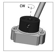
When the marking of the position marker is opposite to the cable outlet, the sensor is located at the reference pulse (Z)
