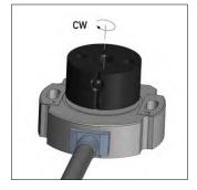
When the marking of the position marker points to the cable outlet, the sensor is located in the electrical center position.
