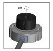
When the marking of the positon marker points to the cable outlet, the sensor is locted in the electrical center position.
