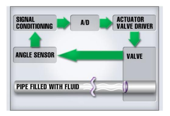
Each component in the application contributes to the error total including the fluid the valve is in contact with through its bulk modulus elasticity. However, closed-loop control can compensate for latent valve movement caused by fluid compression so, except for a small delay, we are left with adding up the tolerances of the angle sensor, signal conditioning circuitry, A/D converter, valve driver circuitry and hydraulic valve.
