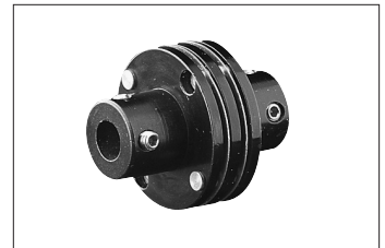
Z 110 G 10 Backlash-free coupling for 10 mm shaft diameter. Black anodized aluminum, driving pin and spring in phosphor bronze. Mounting with 2 threaded pins M 4 each with hexagon socket. Maximum torque 25 Ncm.
