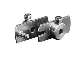
Z 103 G 2.5 Z 103 G 3 Fork coupling with low backlash for 2.5 mm or 3 mm shaft diameters. Stainless steel, ground driving pin. Mounting with 1 fillister head screw M 2 each with hexagon socket. Allen key size 1.5 is supplied.
