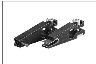
Z 105 G 6 Backlash-free fork coupling for 6 mm shaft diameter. Black anodized aluminum, driving pin and spring hardened. Clamp mounting with 1 fillister head screw M 3 each with hexagon socket. Maximum torque 5 Ncm. Allen key size 2.5 is supplied.
